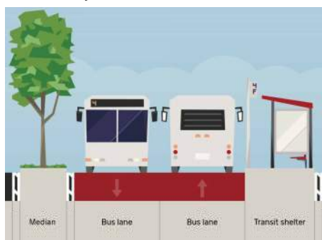
Median layout at BRT station
