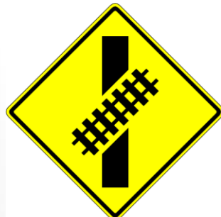
W10-12 Skewed Railroad Crossing
