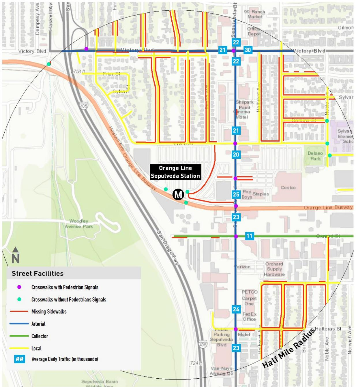
Figure 2: Pedestrian Facilities and Road Types
