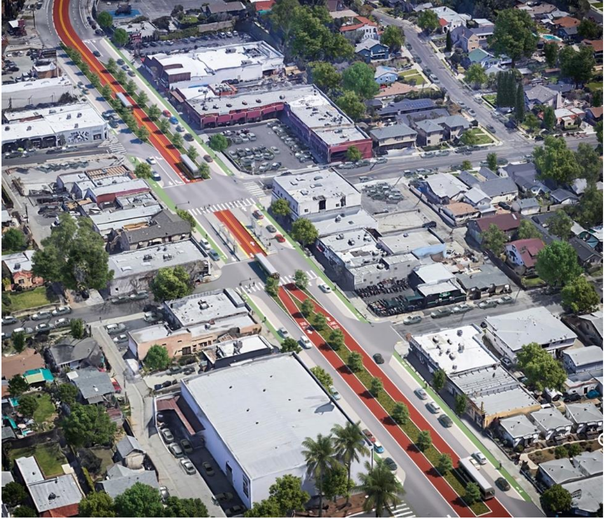
Figure 6: Center-running BRT on Colorado Boulevard in Eagle Rock (east of Eagle Rock Boulevard) – design option with single travel lane (Staff recommendation)
