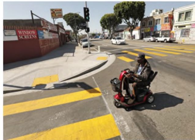
To help reduce fatal traffic crashes, the city of L.A. has added new crosswalks that extend further into the street, such as this one at 43rd and Broadway. (Al Seib / Los Angeles Times)
