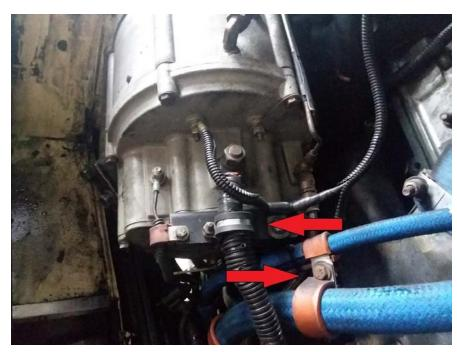
Alternator cable and hydraulic oil line securement
