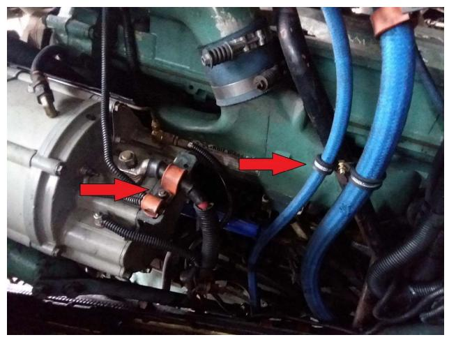
Alternator cable and hydraulic oil line securement
