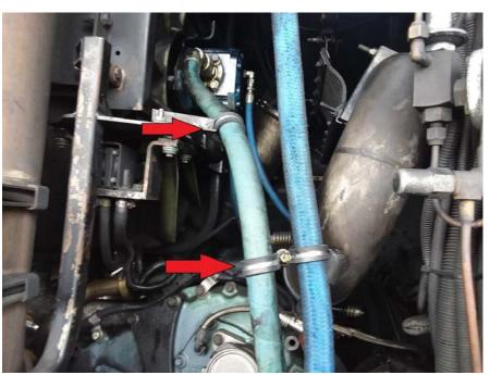
Hydraulic fan oil line securement
