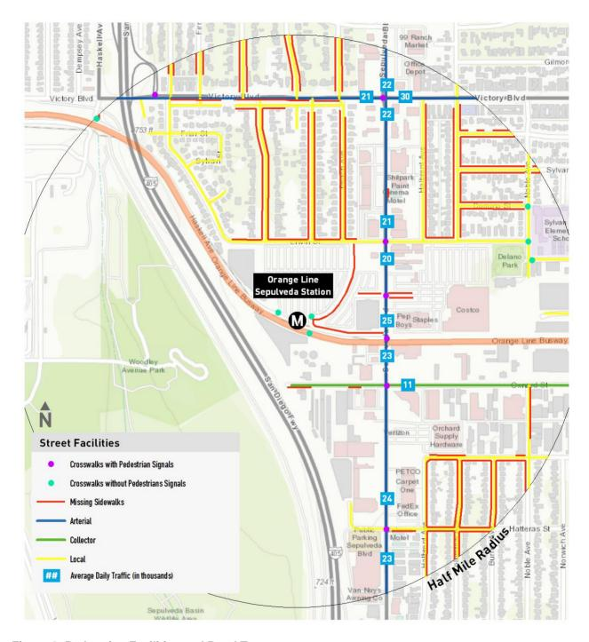
Figure 2: Pedestrian Facilities and Road Types
