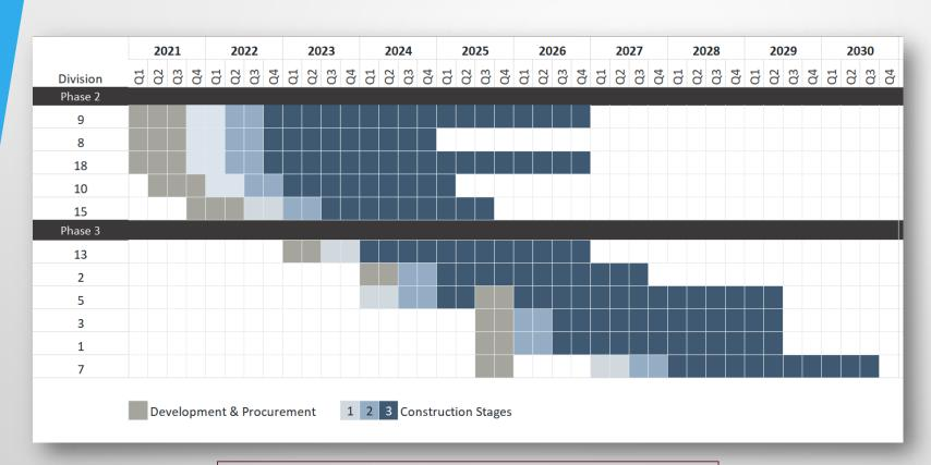
Bus deliveries are timed with completion of construction stages and en-route charging installations.
